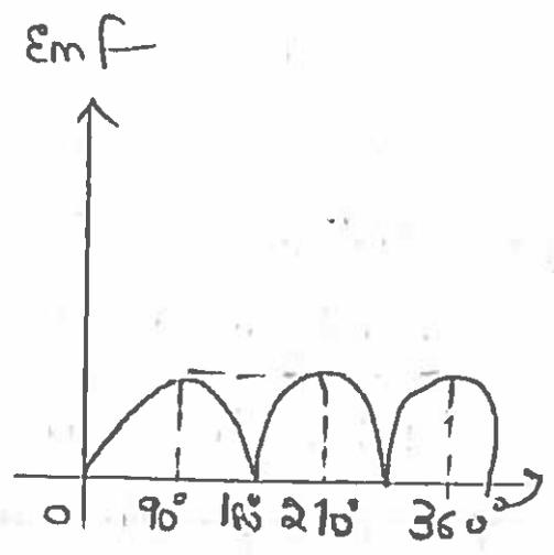
2. commutator is a conducting cylinder which is cutting into two half segments these are insulated from each other by using mica.
