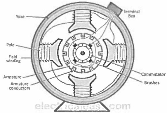
**Yoke:** The outer frame of a dc machine is called as yoke. It is made up of cast iron or steel. It not only provides mechanical strength to the whole assembly but also carries the magnetic flux produced by the field winding.
