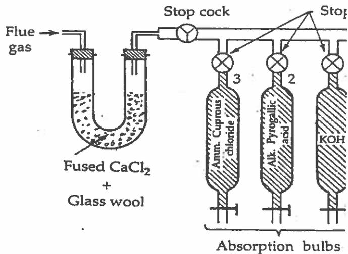
Fig: Orsat's Apparatus
