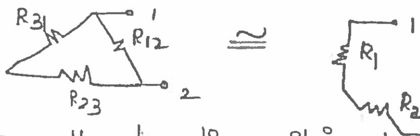
From the above figure it is observed that  $R_{23}$  and  $P_{31}$  connected in series and that combination in parallel with  $R_{12}$ . In star connection  $R_1$  and  $R_2$  are connected in series.
