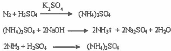
$$\% \text{ of N}_2 = \frac{\text{Volume of acid} \times \text{Normality of acid} \times 1.4}{\text{Weight of coal taken}}$$
