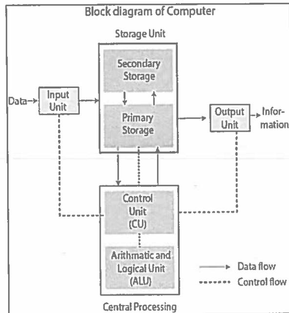
**Computer Block Diagram System:** Mainly computer system consists of three parts, that are central processing unit (CPU), Input Devices, and Output Devices. The Central Processing Unit (CPU) is divided into two parts again: arithmetic logic unit (ALU) and the control unit (CU). The set of instruction is in the form of raw data.
