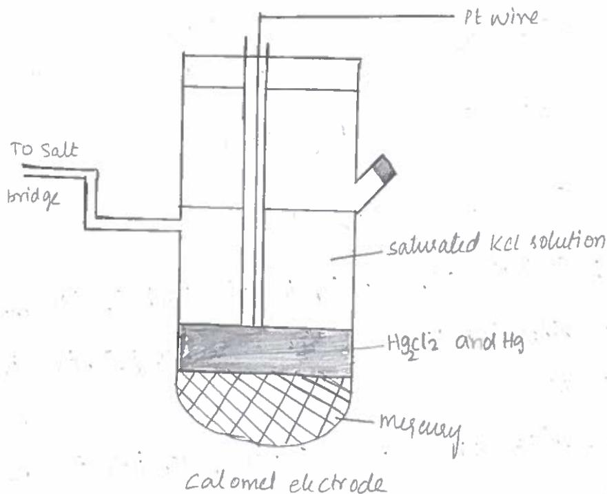
Calomel electrode is a metal-metal salt ion electrode. It consists of mercury, mercurous chloride and a solution of KCl. Mercury is placed at the bottom of a glass tube having a side tube on each side. Mercury is covered by a paste of mercurous chloride (calomel) with mercury & KCl.
