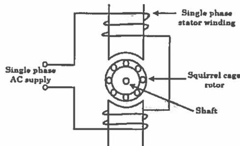
Principle of operation of single phase induction motor:
