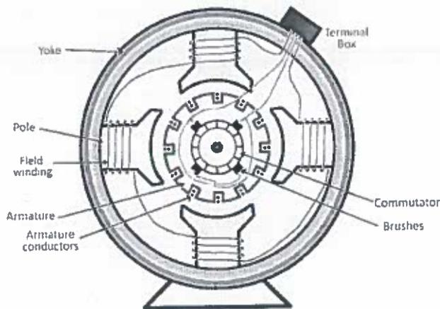
Figure : constructional details of a simple 4-pole DC machine.
