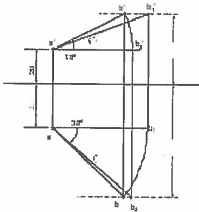
The line AB of 40mm length is inclined at  $30^\circ$  to the H.P. and  $60^\circ$  to V.P. The end point A of the line is 15mm above H.P. and 20mm in front of V.P. Draw the Projections of lines?
