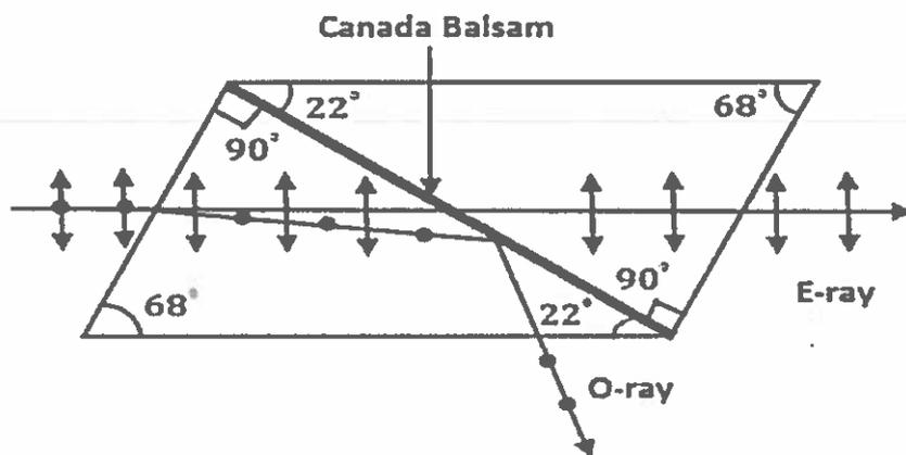
**Working:** When an unpolarized light incident on Nicol prism, it splits into two rays Extraordinary ray and ordinary ray. Both the rays are plane polarized. Because of construction of Nicol prism, the ordinary ray incident on the Canada Balsam interface at angle greater than critical angle and suffers total internal reflection. The extraordinary ray transmitted through Canada Balsam and emerges out of the prism. In this way plane polarized light is obtained.
