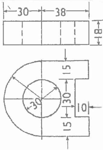
12 Draw the isometric view of considering the orthographic projections shown in figure.
