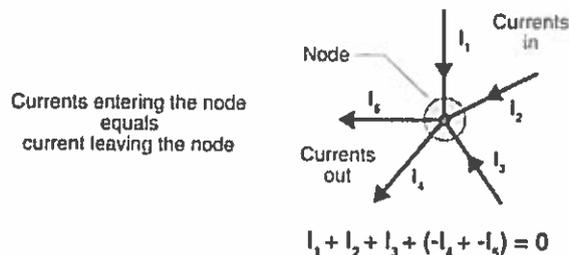
In the above figure, the currents  $I_1$ ,  $I_2$  and  $I_3$  entering the node is considered positive, likewise, the currents  $I_4$  and  $I_5$  exiting the nodes is considered negative in values. This can be expressed in the form of an equation:
