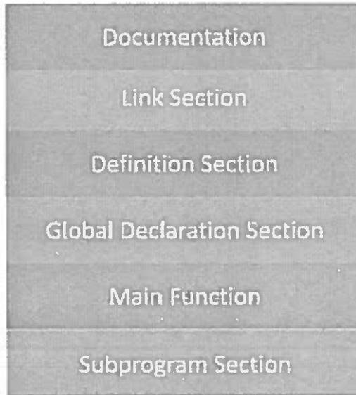
Figure: Basic Structure Of C Program
