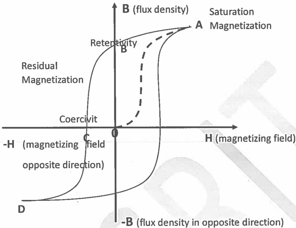
The area of the hysteresis loop gives the loss of energy due to the cycle of magnetization and demagnetization and is dissipated in the form of heat. The retentivity and coercivity of the hysteresis loop are the characteristics of different ferromagnetic materials.
