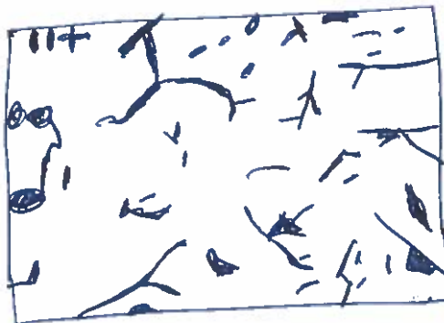
Gray iron showing graphite flakes (black) and ferrite (white portion)
