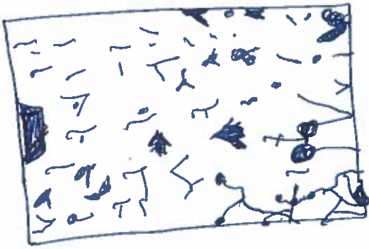
Ferritic malleable iron showing ferrite matrix and temper carbon (dark particles)
